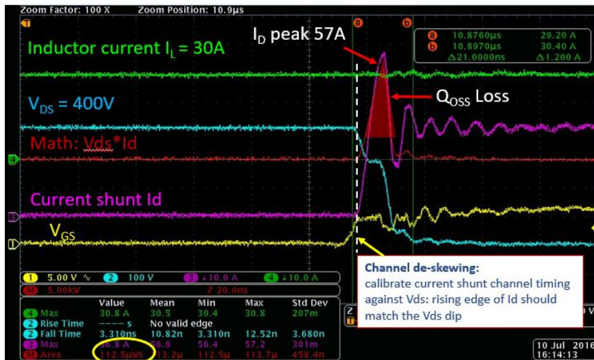
Figure 20 Turn-on switching loss measurement ( E_{on}=113\mu J , 400V/30A)
