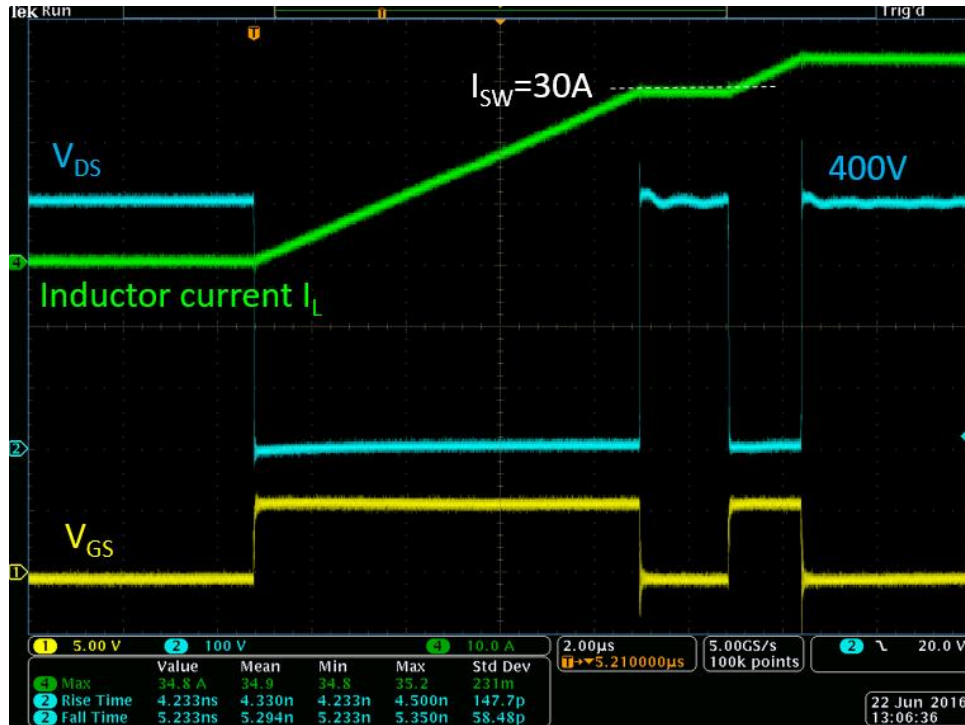
Figure 16 400V/30A double pulse test waveform
